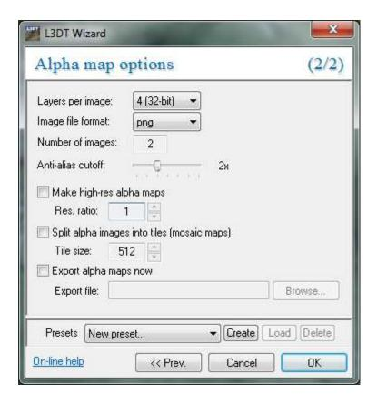
This wizard pane wizard pane allows you to set various parameters that affect the size and format of the alpha maps. In T3D, the alpha map must be the same size as the heightmap. This means that you must leave the *make high-res alpha maps* option **unchecked**, with the *res. ratio* value set to 1, as shown above.
