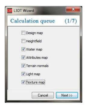
Click 'next »' to proceed to the *water map* wizard pane. Whilst T3D does support multiple water bodies at different levels using 'water blocks', it is rather difficult to set up and get right. Thus, it is recommended that you disable the 'auto flood seas' and 'auto flood lakes' options, and instead enable the 'flood water plane' options (as shown below). This will create one water level for your map.
